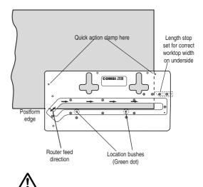
Ensure the router base does not foul the jig body at the end of the replaceable insert recess.
