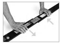
Put two plastic spacers onto each bradawl blade. Take care of the sharp point. When using bradawls always ensure the two spacers are fitted.
