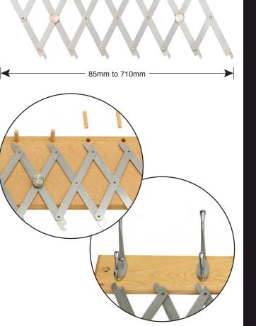
Simply expand the point to point mechanism, find the ideal spacings and lock the 7-point marking positions. then transfer to component.
